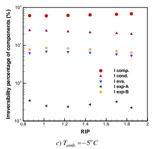
Fig. 4 Percentage of the Total irreversibility created of the components of the system at various ambient temperatures.
