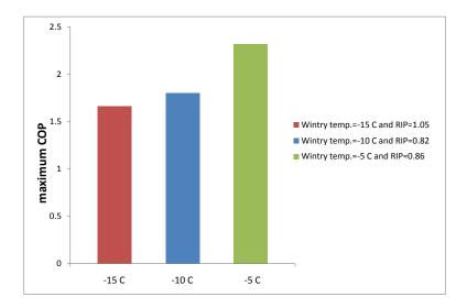
Fig. 10 Maximum COP condition of the HPSCSC at various ambient temperatures.
