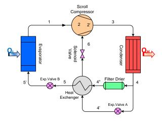
Figure 1. Heat pump system with economizer.
